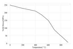
Figure 2. Variation of Yield Strength with Temperature
