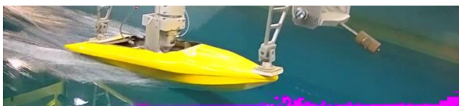
Fig. 10. Model under test with trim tab A at a speed of 3 meters per second
