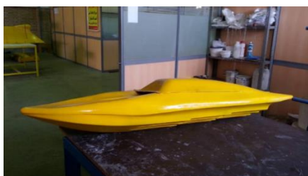
Fig. 6. Photograph of the completed hull model
