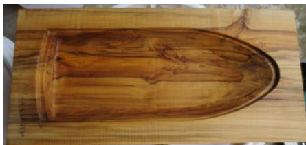
Fig. 5. Initial mold used for hull model construction
