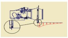
Fig. 2. Interceptor control system installed on the hull bottom [3]
