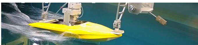
Fig. 11. Model under test with trim tab size A at a speed of 4 meters per second
