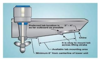
Fig. 1. Main components of a trim tab
