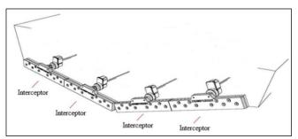
Fig. 3. Hull bottom equipped with four interceptors [15]
