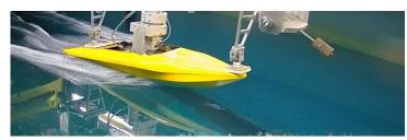
Fig. 7. Model Testing Without Trim Tabs at 2 m/s
