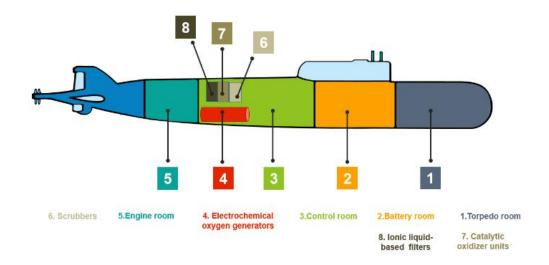
Figure 4. A submarine model showing the location of the filters and generators.
