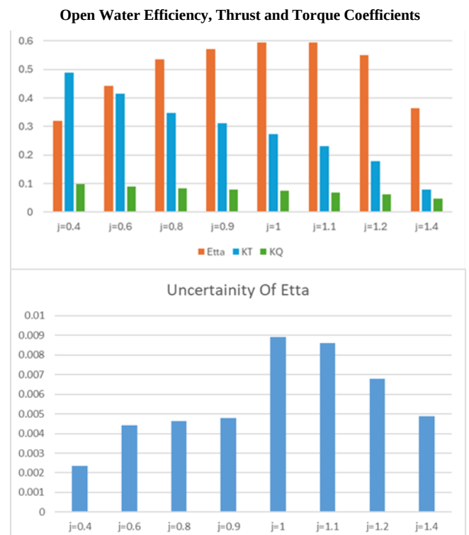
Figure 8: Bar chart arrangement. Up to down: Efficiency plot, thrust and torque coefficients, open water efficiency uncertainty plot, Open water efficiency values with upper and lower bounds; relative uncertainty plot for duct and stator thrust, rotor thrust, total thrust, rotor torque, and open-water efficiency parameters (in percentage terms) across different advance ratios for the L=0DR configuration.
