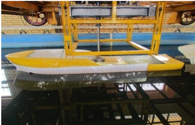
Figure 3. Ship model attached to dynamometer
