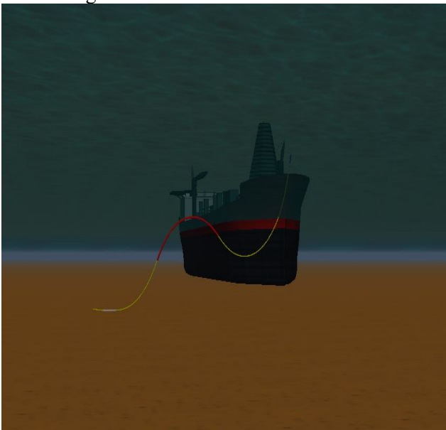
Figure 3. Lazy wave configuration modeling in orcaflex software in the loaded condition
