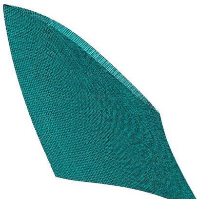
Figure.29 Grid generated on the rotor blades
