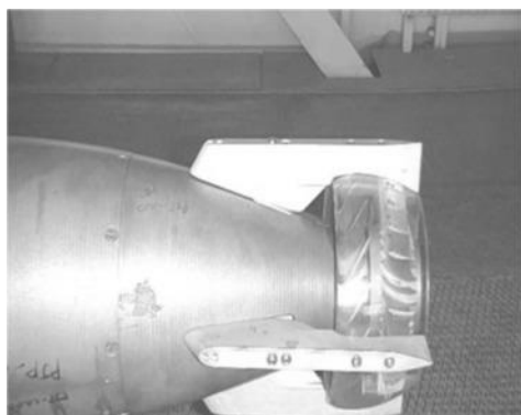
Figure.1 Pump jet propulsion of underwater marine vehicle[1]
