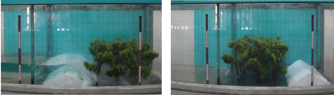
Figure 1- Tree-structure arrangement in the laboratory flume
