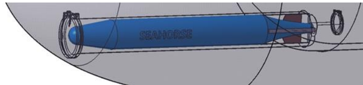
Fig 23. Position of SEAHORSE in the bow horizontal large tube
