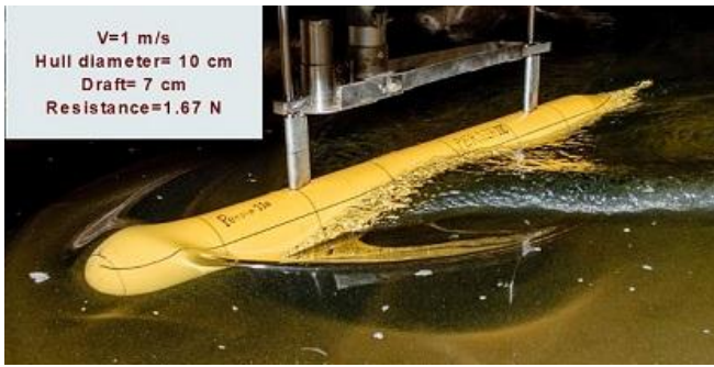
(a) Test in the surface draft of 7 cm and speed of 1 m/s
