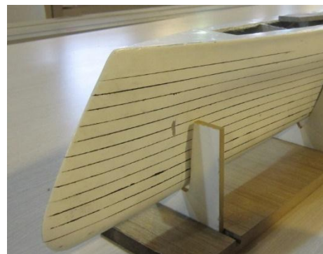
Figure. 1 The centre (main) hull's wave piercing bow profile
