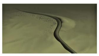
Figure 1. Schematic diagram of lateral buckling in offshore pipeline [13]
