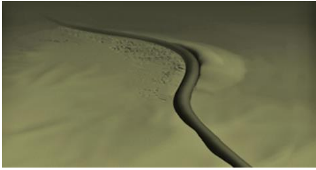
Figure 1. Schematic diagram of lateral buckling in offshore pipeline [13]
