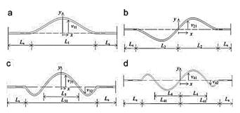
Figure 2. Buckling mode shapes [4]
