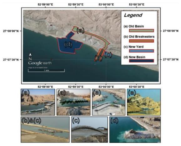
Figure 2. Locations and pictures of; (a): old basin of the port established in 1984, (b): breakwater arms of the old basin modified in 2001, (c): new port yard constructed in 2005, (d): new breakwater arms and basin constructed in 2011.
