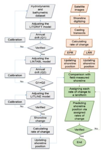
Figure 4. Workflow diagram of the research. The purple and the orange colored shapes represent the modeling procedure of the numerical method and the historical trend method, respectively.
