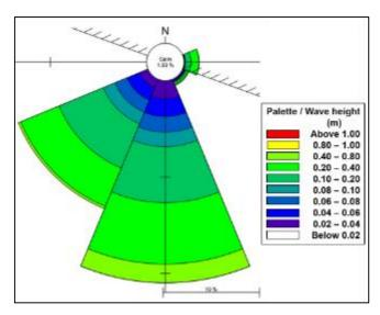
Figure 7. Rose-plot of the area. It represents the condition of wave height distribution relative to the wave direction for the years 1999 to 2006.
