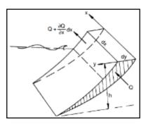
Figure 6. The section for developing sediment continuity equation [14].
