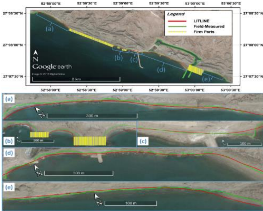
Figure 10. Result of LITLINE simulation in comparison with the field-measured shoreline. Both shorelines are associated with end of 2009. The background image is related to the available satellite imagery by closest date to the year 2009 (i.e. 10/09/2011).
