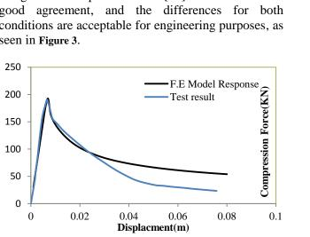
Figure 2. Verification of Brace Behavior
