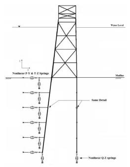
Figure 4. Pile-Soil System Modeling in OpenSees
