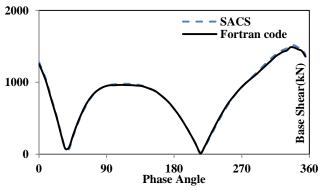
Figure 3. Verification of Wave Force Generation
