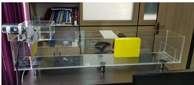
Figure 1. Small portable wave flume with vertical seawall and the overtopping measurement tank and the top-hinged flap and the electric motor.
