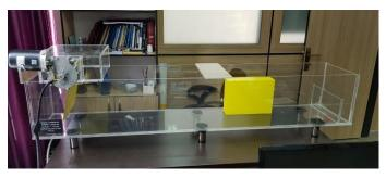
Figure 1. Small portable wave flume with vertical seawall and the overtopping measurement tank and the top-hinged flap and the electric motor.
