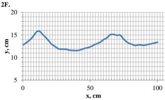
Figure 2. Input waves; water surface from high-speed images has been captured using web-based image processing software [12]
