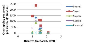
Figure 3. the measured wave overtopping
