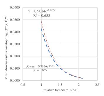
Fig. 6. Comparison between Owen's formula and test data for the slope structure 1:1.5
