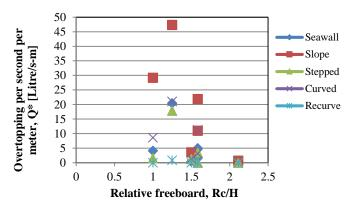
Figure 4. Wave overtopping in prototype scale
