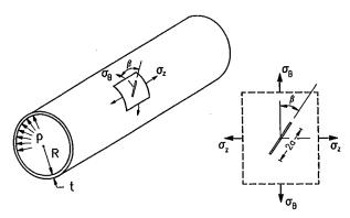
Figure 9. Through-cracked cylindrical pressure vessel [17].
