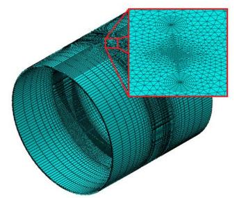
Figure 10. Finite element mesh for a through-cracked cylindrical pressure vessel.
