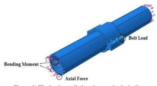
Figure 8. The loads applied to the repaired pipeline.
