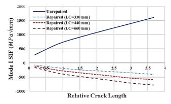
Figure 5. Crack response for the repaired pipeline (Inclined cracks with inclination angle 45°).
