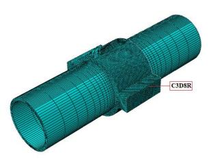
Figure 6. Finite element mesh for repaired pipeline.
