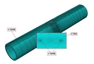
Figure 5. Finite element mesh around an inclined crack.
