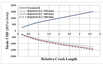
Figure 6. Crack response for the repaired pipeline cracks with inclination angle  $60^{\circ}$ ).
