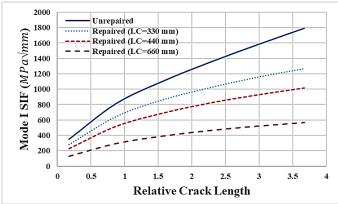
Figure 3. Crack response for the repaired pipeline (Circumferential cracks).
