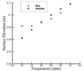
Figure 11 - Validating the wave height outside the OWC for the draft depth of 25 cm
