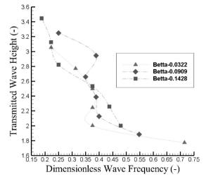
Figure 18 – Prototype transmitted wave height variation by dimensionless frequency
