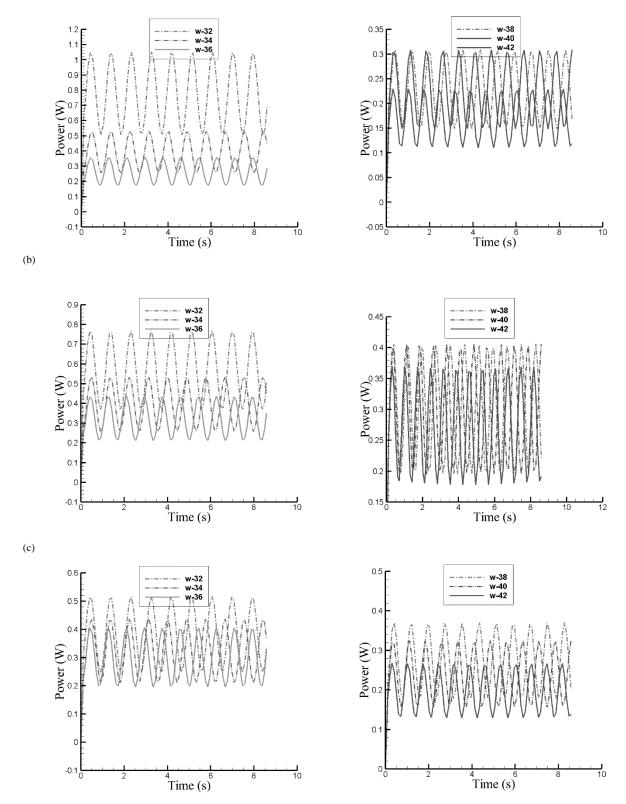
Figure 16 – Output power of the OWC at the draft depth of a)5cm b)15cm c)25cm for various frequencies by time
