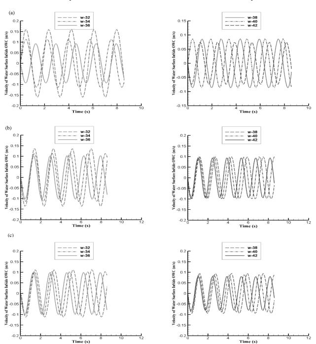
Figure 15 - Water free-surface velocity inside the OWC at the draft depth of a) 5cm b) 15cm c) 25cm for various frequencies by time
