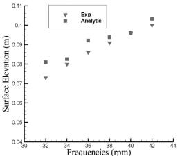
Figure 9 - Validating the wave height outside the OWC for the draft depth of 15 cm
