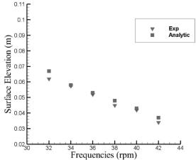
Figure 10 - Validating the wave height inside the OWC for the draft depth of 25 cm
