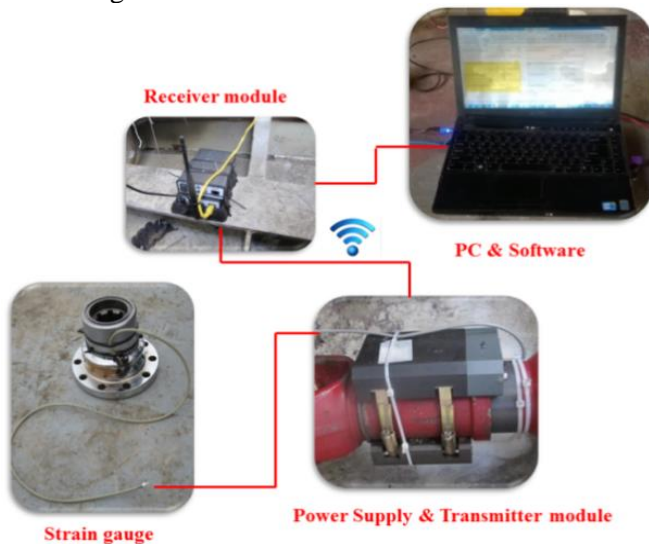
Figure 6. Schematic of torque measuring device
