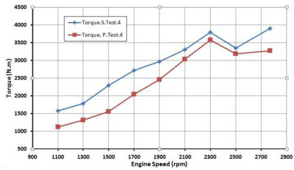
Figure 12. Propeller torque values in the fourth sea trial
