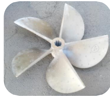
Figure 2. Surface piercing propeller used in this paper
