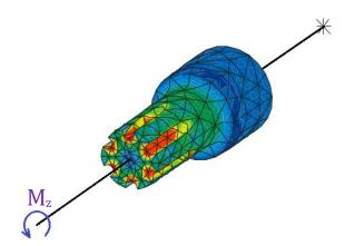
Figure 2- Von Mises stress on 3D model [27].
