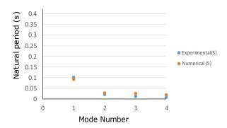
Figure 15- Comparison of the natural periods of the improved facilitated model and laboratory model
