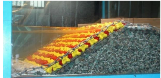
Figure 1 Geometry of breakwater built in the lab [16]
