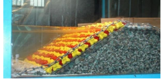
Figure 1 Geometry of breakwater built in the lab [16]
