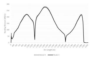
Figure 4. Maximum Bending moment for an SCR and a LWSCR
