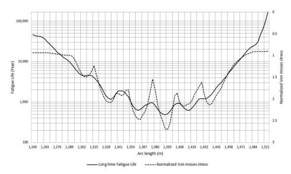
Figure 7. Long time Fatigue life and Normalized von misses stress for Model 1
