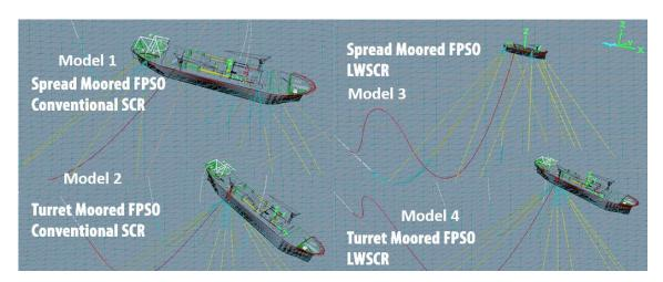
Figure 2. Schematic of mooring and riser models
