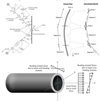
Figure 2. Representation of line FE model and stress distribution
