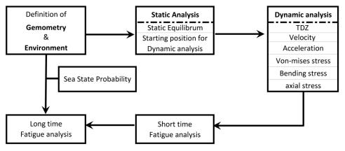
Figure 4. Block diagram of present analysis
