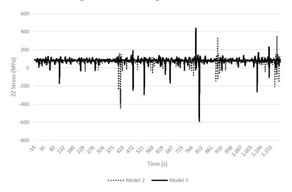
Fig. 5 Axial Stress at the point with maximum bending moment
