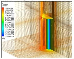
Figure 18. Pressure contours on model 1,  $\Omega$ =4
