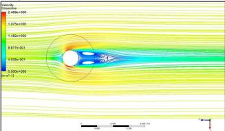
Figure 14. Velocity Streamline for model 1 & 2, plane 6,  $\Omega = 0$
