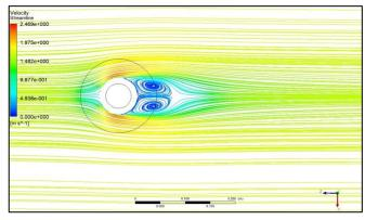
Figure 12. Velocity Streamline for model 2, plane 4 and  $\Omega = 0$
