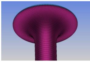
Figure 5. Close view of the structured mesh in model 2
