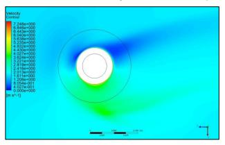
Figure 17. Velocity contours for model 2, plane 4 and  $\Omega = 4$
