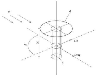
Figure 2. The forces produced on a rotor along with the end disk
