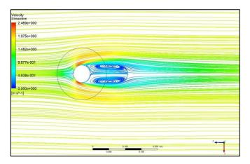
Figure 13. Velocity Streamline for model 2, plane 5 and  $\Omega = 0$
