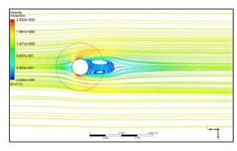
Figure 11. Velocity streamline for model 1, plane 4 and  $\Omega = 0$
