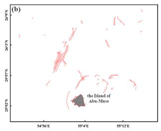
Figure 2. Internal waves on Landsat 7 on May 19, 2000 around the Island of Abu-Musa in the Persian Gulf (a), Result of edge detection algorithm on the related image (b).
