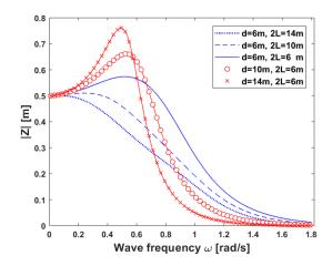
Figure 7. The variation of water level displacement at different sizes of the chamber
