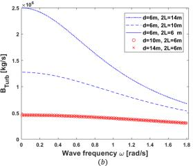
Figure 3. The variation of the induced a) virtual mass and b) damping of the turbine versus frequency at the different sizes of the chamber
