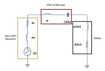
Figure 4. Equivalent RLC circuit model for the OWC
