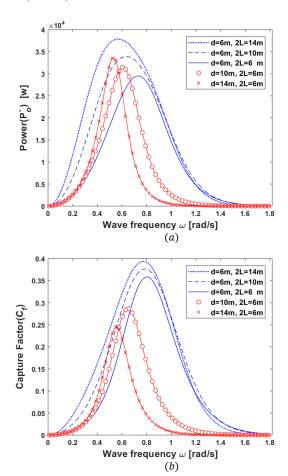
Figure 9. The variation of a) the output power and b) the capture power versus frequency at different chamber sizes
