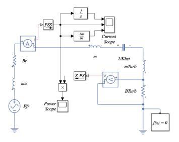
Figure 5. Equivalent electrical circuit model in Matlab Simulink
