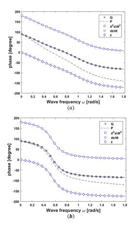
Figure 10. The variation of the phase of variables versus frequency for the case with a) d=6m, 2L=14m, and b) d=14m, 2L=6m
