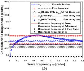
Figure 16. The Comparison of the characteristic frequencies for cases with a) d=10m, 2L=6m, and b) d=14m, 2L=6m
