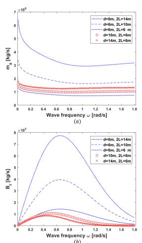
Figure 2. The variation of a) added mass and b) radiation damping versus frequency at the different sizes of the chamber
