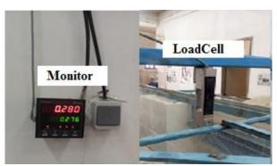
Figure 2- Electronic dynamometer
