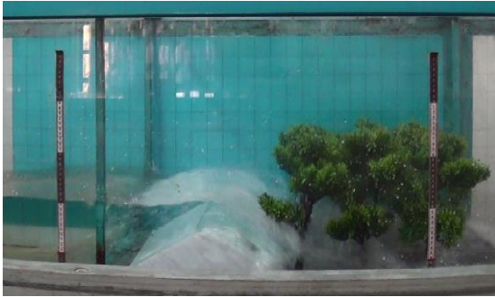
Figure 1- Tree-structure arrangement in the laboratory flume
