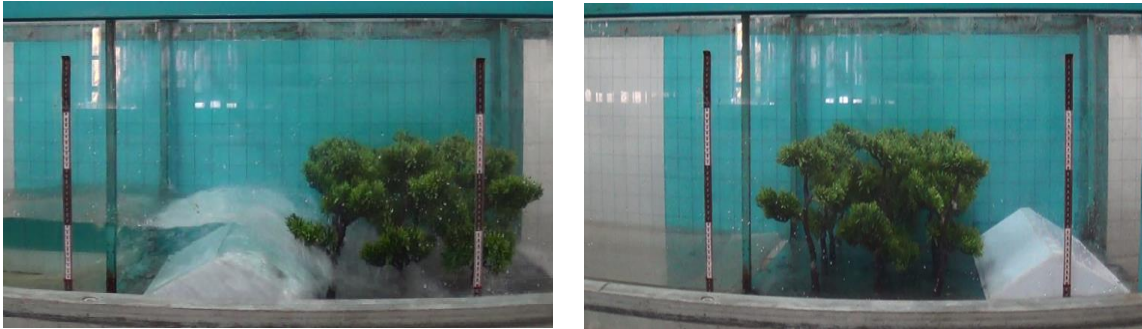
Figure 1- Tree-structure arrangement in the laboratory flume
