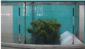
Figure 1- Tree-structure arrangement in the laboratory flume
