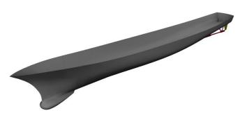
Fig 1. The DTMB 5415 geometry [24].
