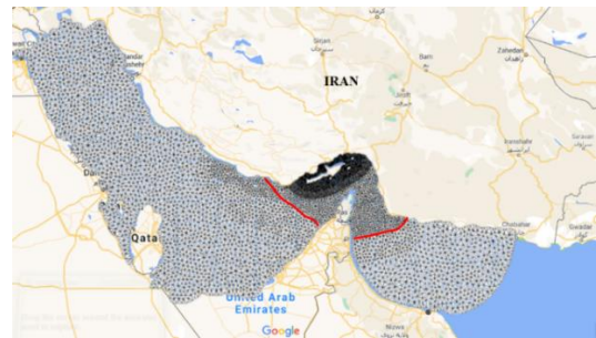
Fig. 7. The domain of the regional model; red lines show the boundaries of the local model
