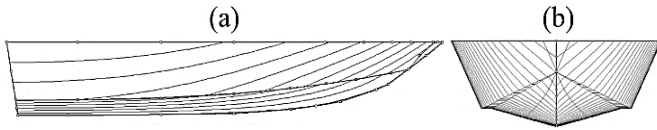
Figure 2. Mono-hull body lines; (a): Right view, (b): Front view
