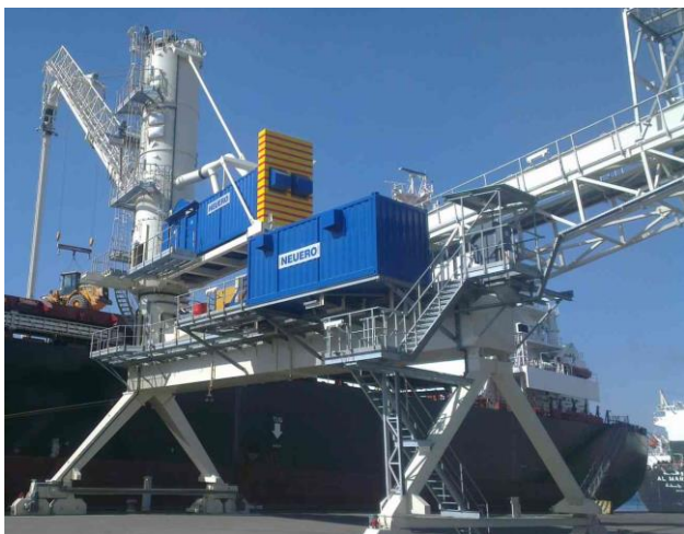
Fig 1: of a grain suction machine unloading cargo from a ship
