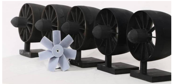
Figure 5: Five Geometries Fabricated for Experimental Testing
