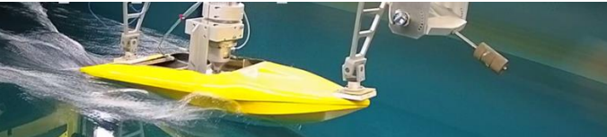
Fig. 11. Model under test with trim tab size A at a speed of 4 meters per second
