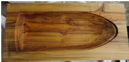
Fig. 5. Initial mold used for hull model construction
